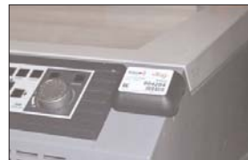
Asset tags communicate with V-Tags that relay information to a host computer.
