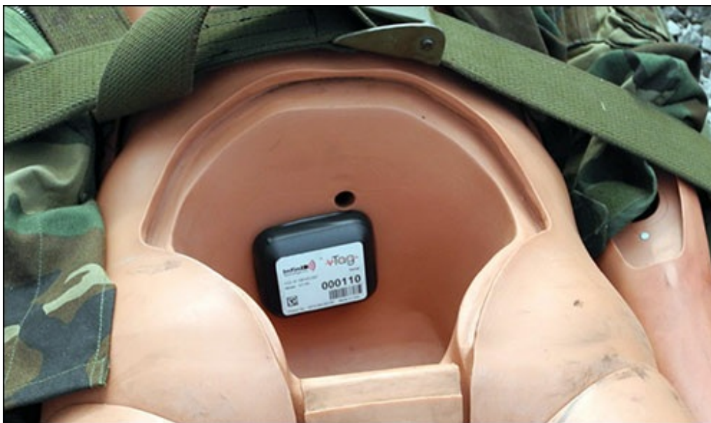
At the Camp Atterbury and Muscatatuck Urban Training Complex, in Indiana, InfinID's V-Tags were placed in manikins representing dead or injured people, which were dispersed around a simulated disaster area as part of training exercises.
